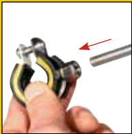
Cropping tongs with 1 pair of reversible cutting inserts for steel, stainless steel, M 6–M 12, up to strength class 4.8 (400 N/mm 2 ).
