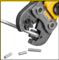
Cropping tongs with 1 pair of reversible cutting inserts for steel, stainless steel, M 6–M 12, up to strength class 4.8 (400 N/mm 2 ).
